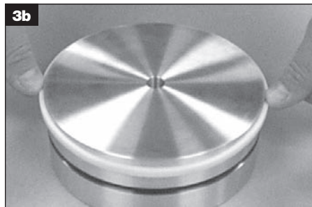
The Piston ring made from modified PTFE material should be stretched minimally to place into the equipment groove. The modified PTFE materials need to be uniformly compressed into the groove. Care should be taken to avoid inconsistent stretching or overstretching.
