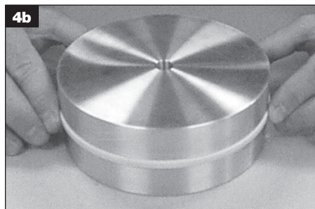
The modified PTFE materials need to be uniformly compressed into the groove.
